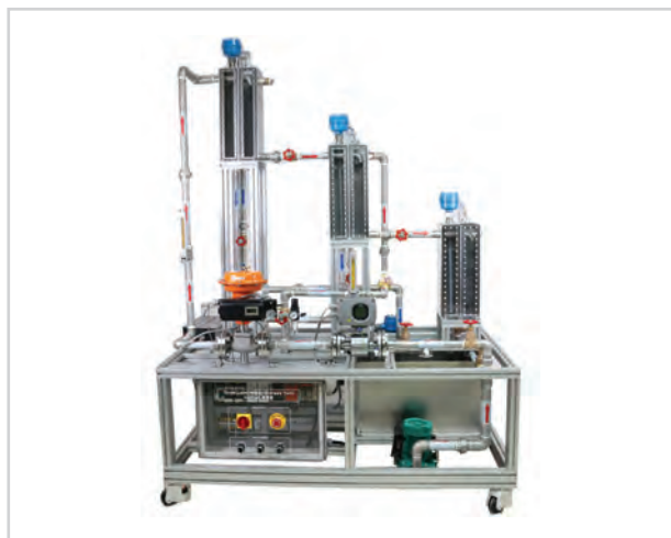
3 tanks control trainer 1600(w)×1000(d)×2250(h) mm
